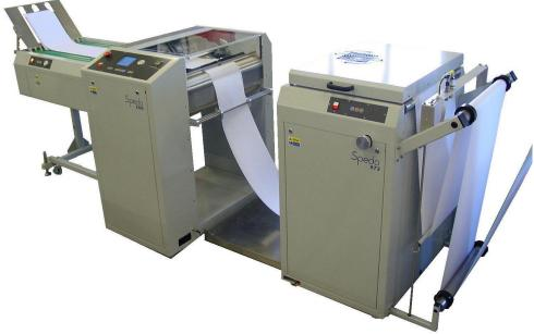
The **SPEDO 973 WEB BUFFER** integrates Spedo systems with your high-speed printer for in-line, print on demand applications, and now includes slit and merge facilities as standard for greater flexibility.
